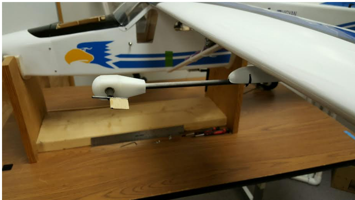
Figure 2.2 Forward Gust Sensor, a.k.a. The Bird
